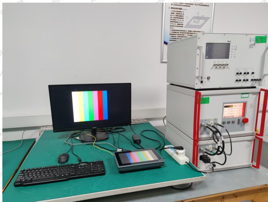
Photo of Electrical Fast Transient/Burst Immunity Test
