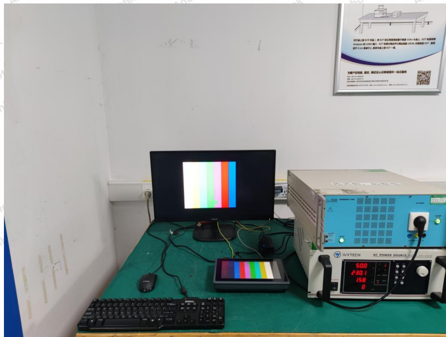
Photo of Harmonic Current And Flicker Test
