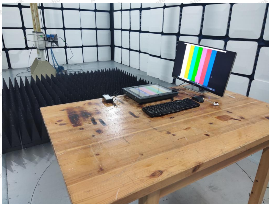
Photo of Radiated Emission Test (Above 1GHz)
