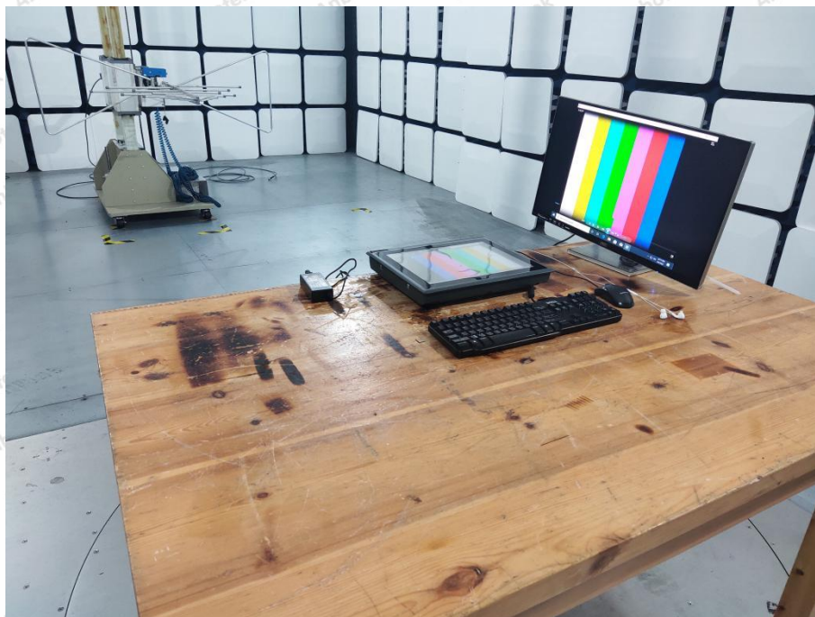
Photo of Radiated Emission Test (Below 1 GHz)
