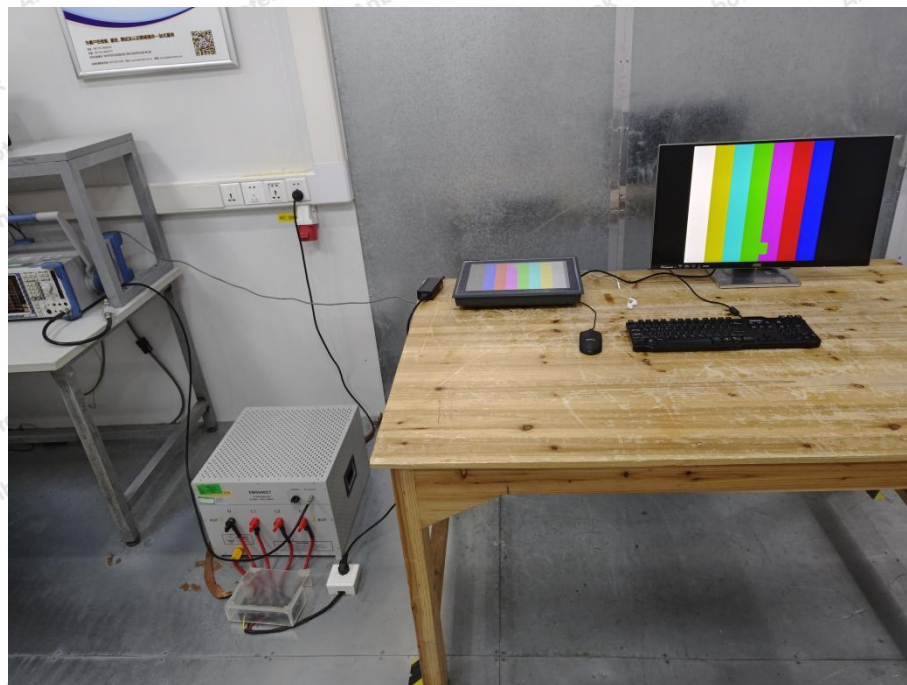
Photo of Power Line Conducted Emission Test
