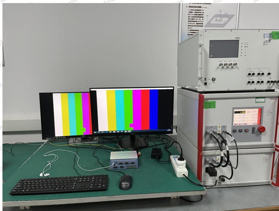
Photo of Electrical Fast Transient/Burst Immunity Test
