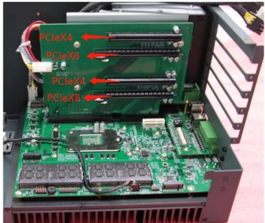
If two GPU graphics cards need to be assembled, the following steps shall be taken to install the video card mounting bracket:
