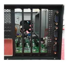
Step 3: Put the PCIe functional module into the expansion slot;
