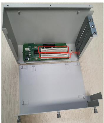
Picture 2.36: PCI installation (3)
