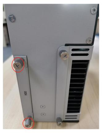
Picture 2.24: HDD/SSD installation (4)
