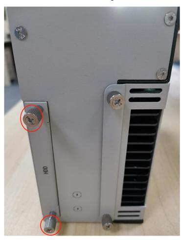
Picture 2.21: HDD/SSD installation (1)
