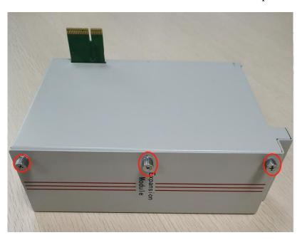
Picture 2.34: PCI installation (1)
