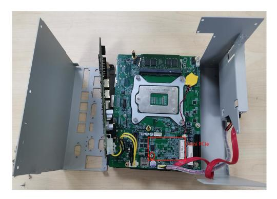
Picture 2.33: Mini PCle installation (1)
