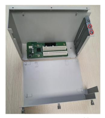
Picture 2.35: PCI installation (2)
