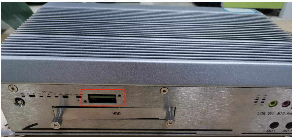
Picture 2.25: SIM1/SIM2 installation (2)
