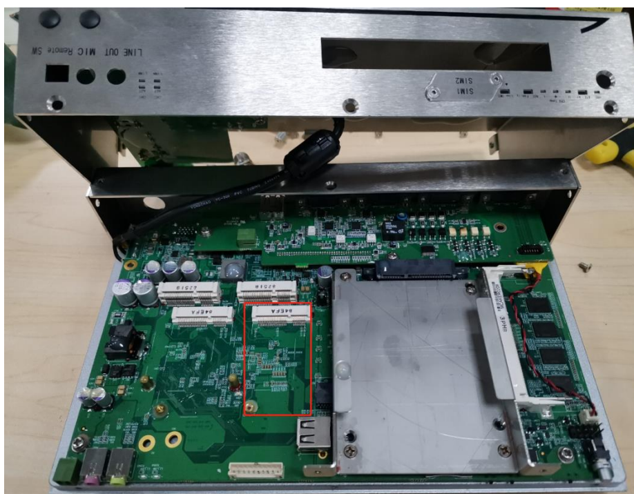
Picture 2.29: mSATA installation (4)
