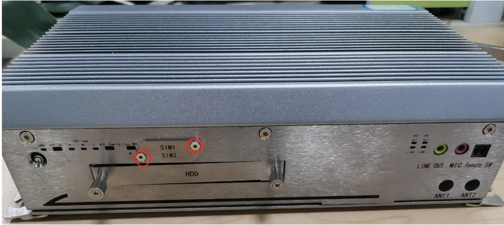
Picture 2.24: SIM1/SIM2 installation (1)
