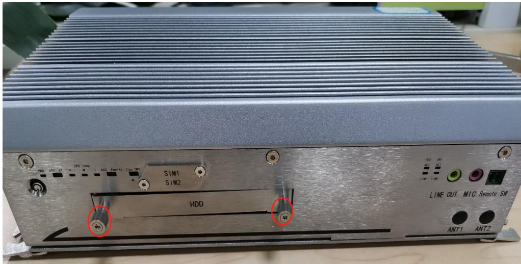
Picture 2.20: HDD/SSD installation (1)
