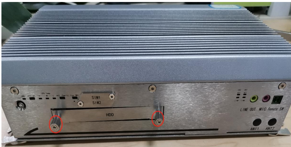
Picture 2.26: mSATA installation (1)
