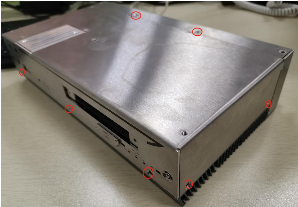
Picture 2.28: mSATA installation (3)
