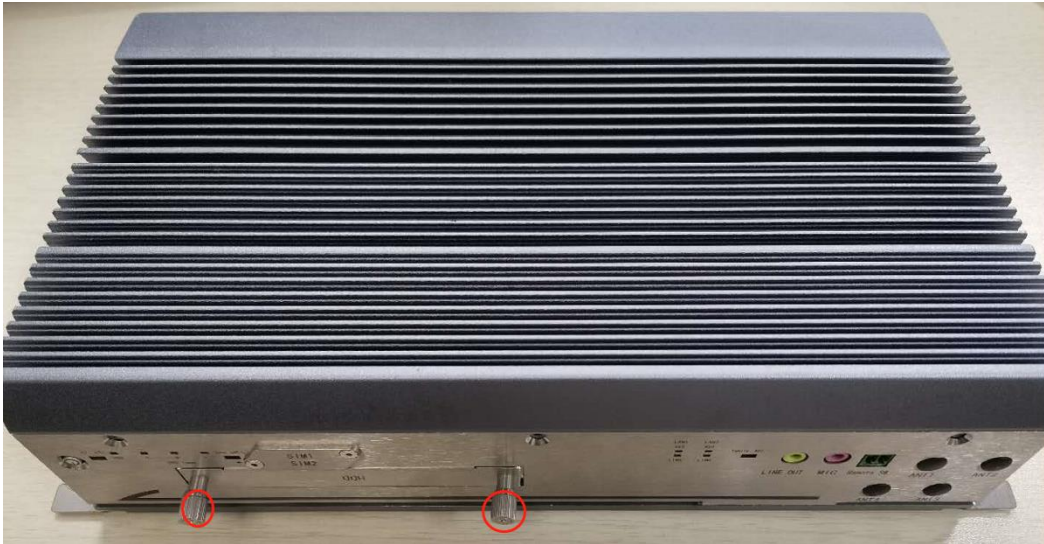
Picture 2.26: mSATA installation (1)
