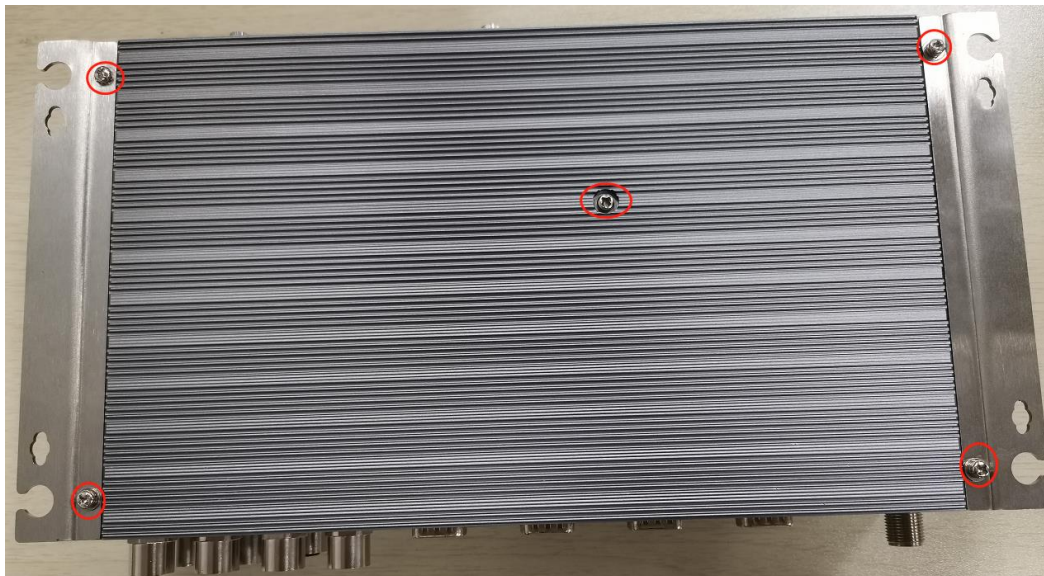
Picture 2.27: mSATA installation (2)
