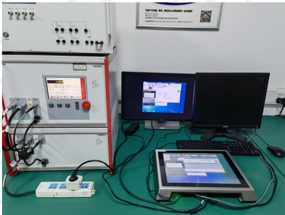
Photo of Surge Immunity Test
